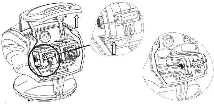
**CAUTION -** Protect the battery contacts when the battery is no longer being used. Loose metal parts may short-circuit the contact - Explosion and fire hazard!
