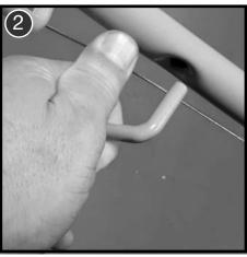
Gently prise the lever inwards from its locating hole in the main handlebar.
