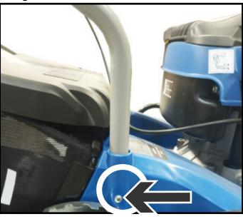
Attach the upper handle to the lower handle and tighten the quick release handle bolts securely. See image 3 & 4.
