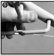
Refit the lever back into its location hole on the main handlebar.
