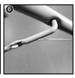
Check the cable lies flat and has not snagged on any other part of the lawnmower.
